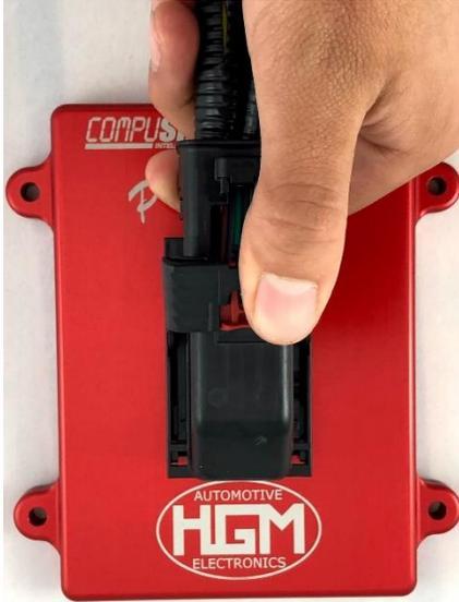
To remove the connector, pull the red tab up, then press down on the release panel.
