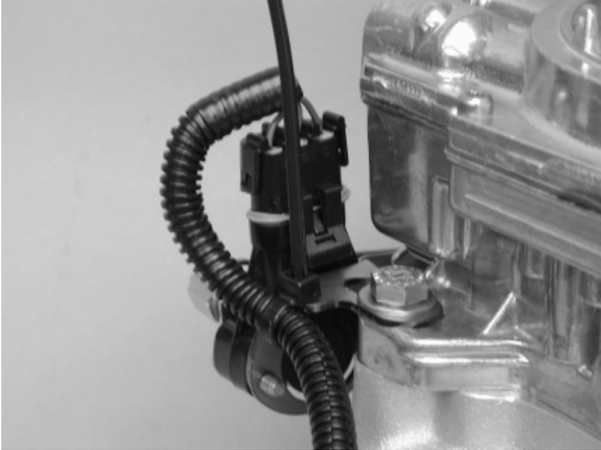
Insert the supplied cable tie from the bottom through the slot in the sensor bracket. Close the cable tie around the wire harness. Cut the excess tie length as desired.
