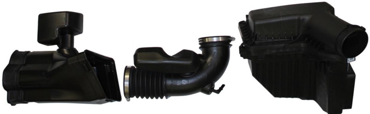
**IMPORTANT NOTE:** The calibration of the PCM you have received requires use of this air box/MAF sensor system exactly as received. Any changes to the air inlet system will result in changes to how the air entering the engine is measured and will require modification to the PCM's calibration.
