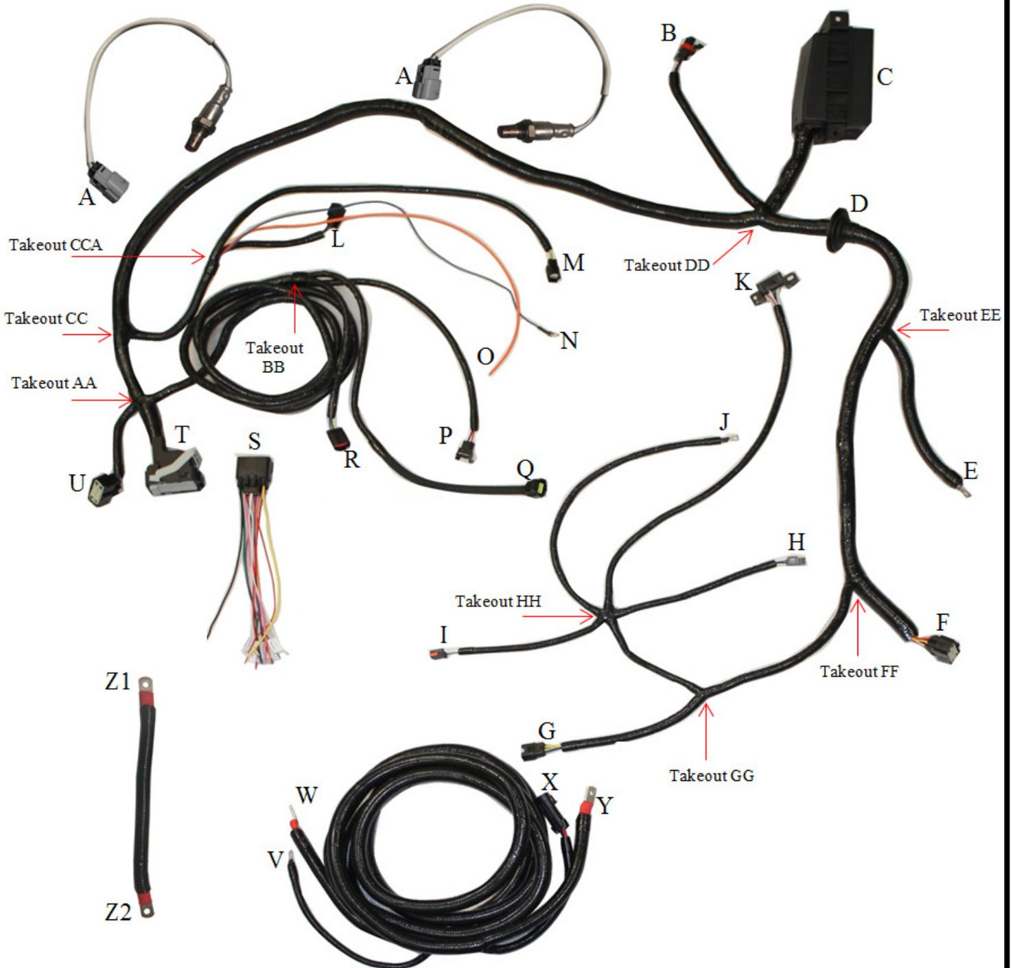
Figure 1 - Controls Pack Wiring Harness Components
