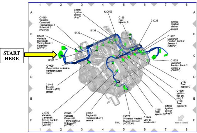
Figure 3 - Rear View of Engine.
