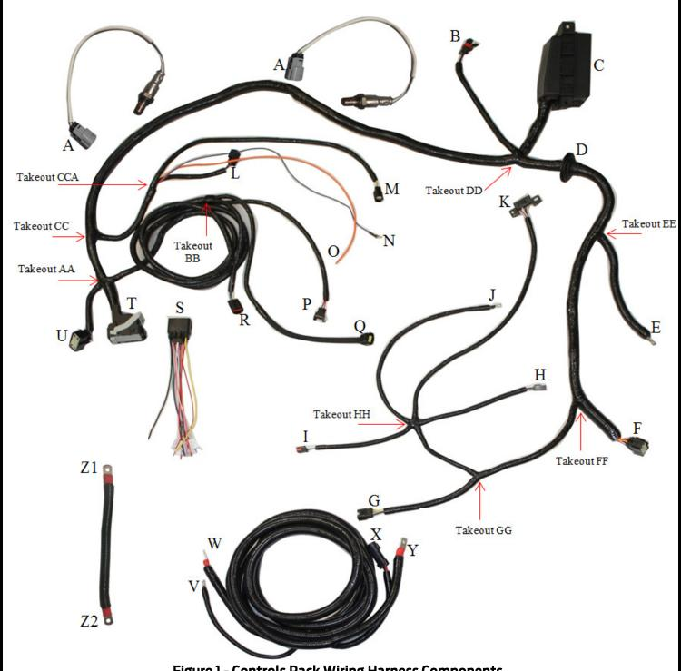
Figure 1 - Controls Pack Wiring Harness Components
